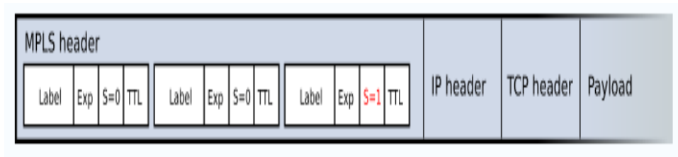
Fig.1.4 MPLS HeaderA 20-bit label value
